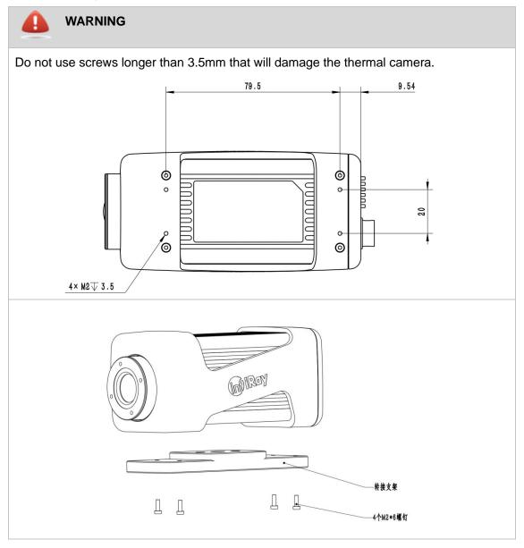
The temperature rise will occur during normal operation. If the thermal camera is used under poor heat dissipation conditions, the temperature rise may be too high, which will affect the temperature measurement performance. In order to ensure the normal use of the thermal camera, it is recommended to be used under good heat dissipation conditions.11.1 Camera Mounting
